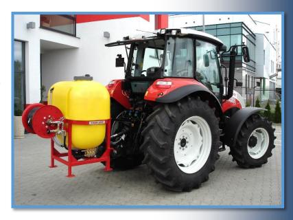
AGROJET high-pressure jetting machin can be mounted on standard agricultural tractor. The device is driven by the agricultural tractor shaft. AGROJET has been equipped with a reliable high-pressure pump from the renowned European manufacturer UDOR from Italy. The pump with ceramic plungers, thanks to which it is possible to work with the device using hot water up to + 70 ° C. It can be one man operated.
